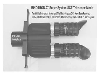
In an SCT (Schmidt Cassegrain Telescope: Simply load the Binotron 27 with only the 2" Nose threaded to the Power Switch into your 2" Star Diagonal Eyepiece Holder. With the Slider of the Power Switch set to "IN" to be very close to "Logo Side" slider arm of the Power Switch pushed in, Reduction .66X will occur and require many counter-Clock wise turns of your SCT Focuser knob. See "Using an SCT" in the Binotron 27 Super System Manual for more details.
