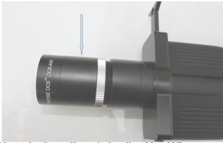
Newtonian Setup: Shown is the adjustable middle spacer. See Manual and "Using in a Newtonian Telescope". See Youtube: "Denkmeier" "Focusing a Newtonian"
