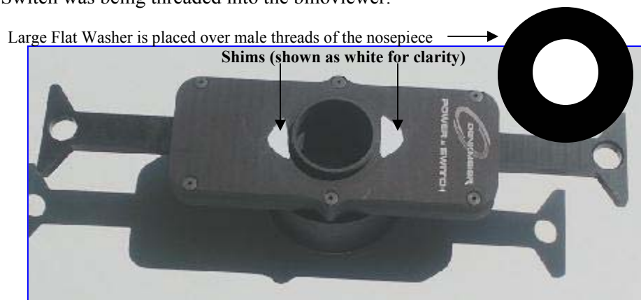
Picture showing location of shim stickers applied to the Dual Arm Power x Switch.
